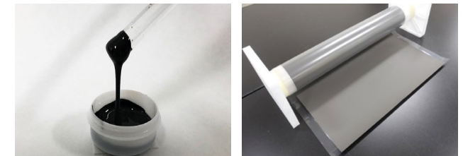
Newly developed magnetic materials (Left) Paste type (Right) Film type
